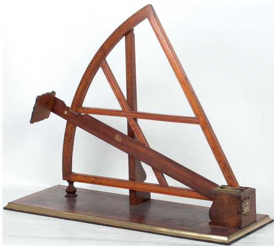
Fig. 1 Instrument to study the refraction index of liquids. Designed by Christian Wolff, it was made for Giovanni Poleni by Philippe Vayringe in the early 1740s. The liquid to be studied was put in the prism container (on the right in the photograph). The light entering through the lateral hole was deviated as it passed through the liquid, and the mobile arm was then moved until the refracted ray of light hit the square wooden piece at the extremity of the arm. Giovanni Poleni Museum, University of Padua.
